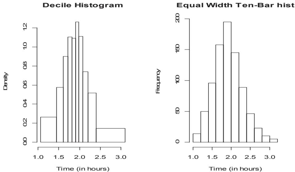
Figure 2. *Left*: Unequal width ten-bar histogram. Classes have limits defined at the deciles. Each bar contains 10% of the data. Special details of the distribution are easily visualized and interpreted.
