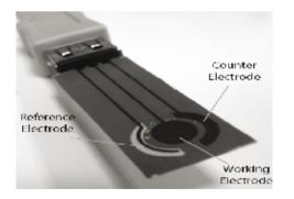
Fig. 5. Photograph of the SPE used in this work.
