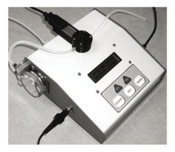
Fig.4. Photograph of the assembled bioamperometer showing the flow cell with the electrode lodged in to perform the analysis. Table 2. Additional technical specifications of the bio-amperometer.
