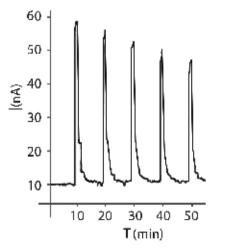
Fig 6. Amperometric measurement performed in static mode on thylakoids from *S. oleracea* immobilized with BSA-GA on a screen-printed electrode. Atrazine is added at intervals of 10 min at 4 different concentration  $(10^{-9}, 5 \times 10^{-9}, 10^{-8} \text{ and } 5 \times 10^{-8} \text{ M})$  starting from 20 min. *Buffer* (pH 7.2): tricine (20 mM), MgCl<sub>2</sub> (5 mM), sucrose (70 mM), NaCl (50
