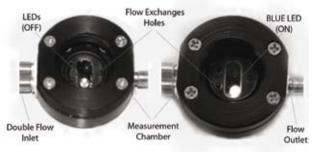
Fig.2. Image of the biosensor cell with one of the two LEDs on. Two flow inlets are provided for mixing solutions or administrating stimuli.
