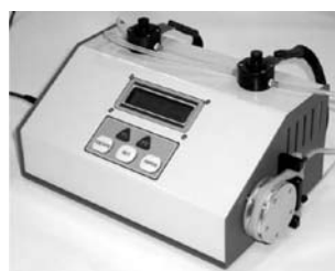
Fig. 5: Picture of the amperometric biosensor is shown in a photograph with two flow cells for biomediators in series.
