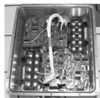
Fig. 4: Picture of the optical biosensor instruments at the end of fabrication, showing the electronic control and measure boards and the optical modules with the LEDs on (right side). The biological containers arrays to be settled over the optical modules are still unmounted.
